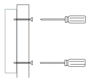
Please note: If the screws become a bit loose while using Stick, please tighten the screws for securing Stick. This way you prevent the drilling holes getting wider.
